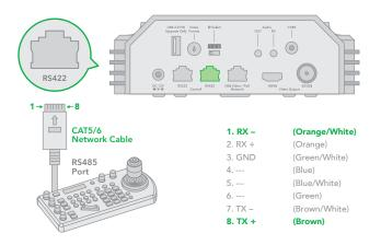
• How to make RS485 multiple cameras connection with RS485 standard serial port controller:
