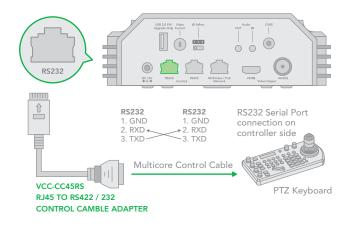
Or you can use CAT5/6 network cable (T-568B standard pinout) to make RS232 connection by following the pin definition below:
