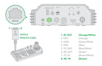
12. How to make RS232 Daisy Chain multiple camera connection with standard RS232 serial port controller as below:
