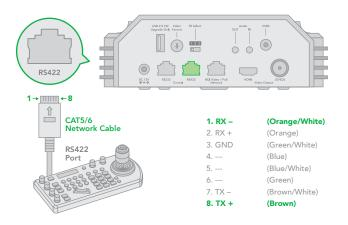
13. How to make RS422 Daisy Chain multiple camera connection with RS422 standard serial port controller:
