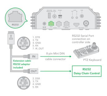
Use extension cables included RJ45 to RS422/232 Phoenix terminal contact adaptor to make RS232 connection for your control device.
