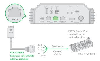
Or you can use CAT5/6 T-568B Standard Ethernet cable direct connect between the camera and the controller to make RS422 connection by following the pin definition below:
