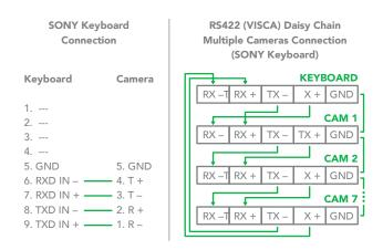
10. How to make RS422 connection and RS422 Daisy Chain multiple cameras connection with Non-Sony controller as below:
