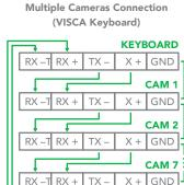
11. Use extension cables RJ45 to RS422 Phoenix connecter adaptor included to make RS422 connection for your control device.
